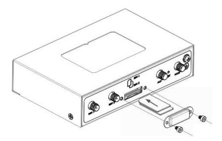
Insert or remove the SIM card as shown in the following steps.
