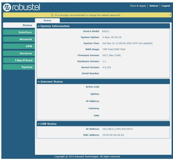
From the homepage, users can perform operations such as saving the configuration, restarting the router, and logging out.
