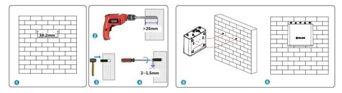
First, drill holes on the wall, the distance between the two holes is 60mm, then knock the expansion pipe into the wall with a rubber hammer, align the screw with the expansion pipe, insert the screw and reserve the corresponding length, and finally fix the product on the wall.
