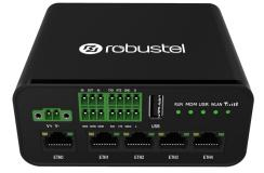
• 1 x 2-pin 3.5 mm male terminal block with lock for power supply
