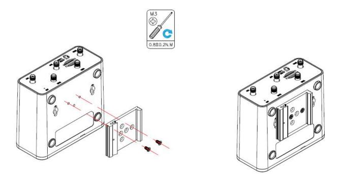
Use 3 pcs of M3\*8 Black cross recessed countersunk head tapping screws to mount the router on the DIN rail, and then hang the DIN rail on the holder. You need to choose a standard holder. **Note:** Recommended torque for mounting is 0.8 N.m, and the maximum allowed is 1.0 N.m.
